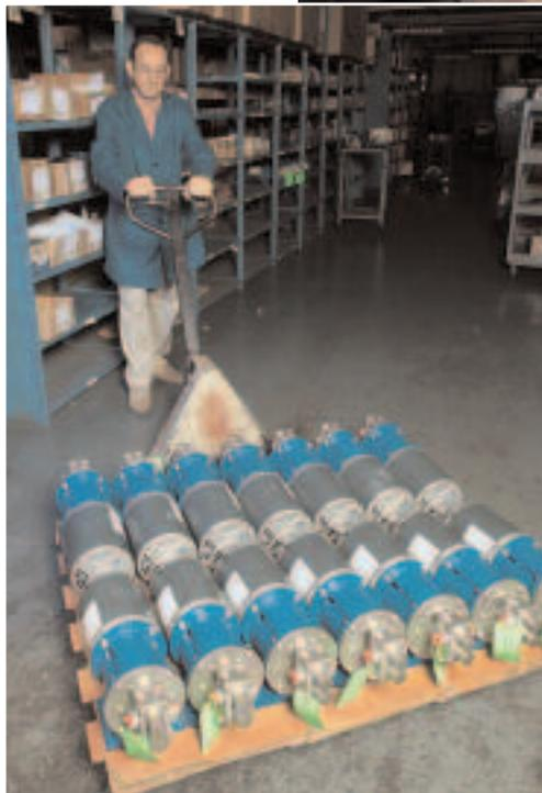
Large order of gear pumps close-coupled to electric motors going to OEM factory: Liquiflo pumps are available with a large selection of ancillary options and accessories. These include flanged ports, relief valves, temperature control jackets, variable speed drives, gear reducers, air motors, base plate mounting and more.
