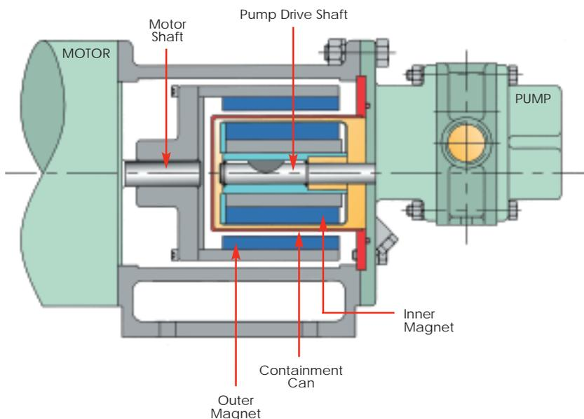
Mag-drive pumps transfer power from the motor shaft to the pump drive shaft via a magnetic coupling. The magnetic coupling consists of an outer magnet and inner magnet, matched in strength. The outer magnet attached to the motor shaft causes the inner magnet attached to the pump drive shaft to turn synchronously with the motor. Since the drive shaft is completely inside the pump housing, there is no need for a dynamic seal and the pumped liquid is completely contained.
