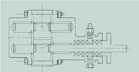
FIG. 1 PACKING SEAL
