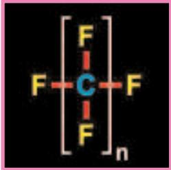
Perfluorocarbon (PFC) coolants are a popular alternative to environmentally hazardous chlorinated solvents. One specialty application for PFC coolants is in high-performance chillers used for stringent semiconductor applications. The chiller systems require highly reliable temperature control, so every part of the system must be absolutely dependable.
