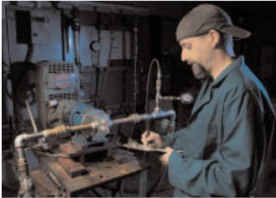
All functional products – including pumps, replacement cartridges and relief valves – are performance-tested before shipping. Testing is performed in accordance with Hydraulic Institute standards.
