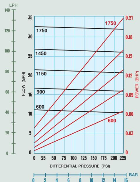
**4-SERIES LOW-FLOW GEAR PUMP
