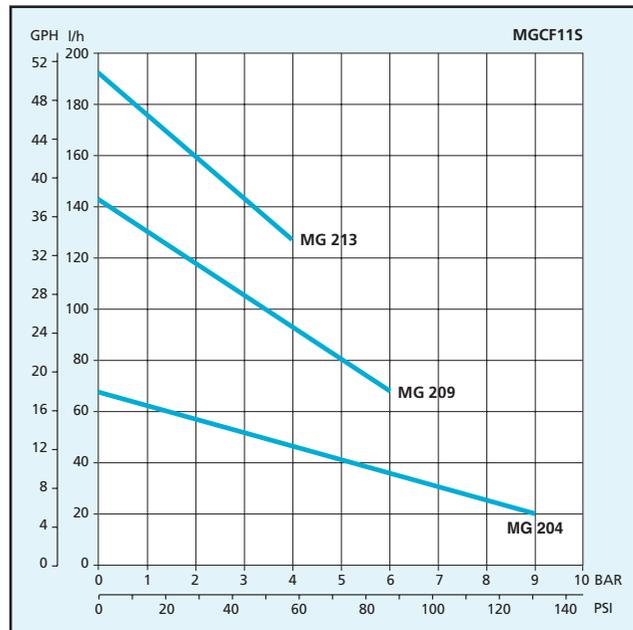
Notes: Characteristics with water at 20 °C (68 °F) and without relief valve, max vacuum 724 mmHg. Use filter before pump inlet not larger than 10 micron. Pump weight: 960 g (2,12 Lbs). Temperature requirements different from ambient temperature must be mentioned on the order.
